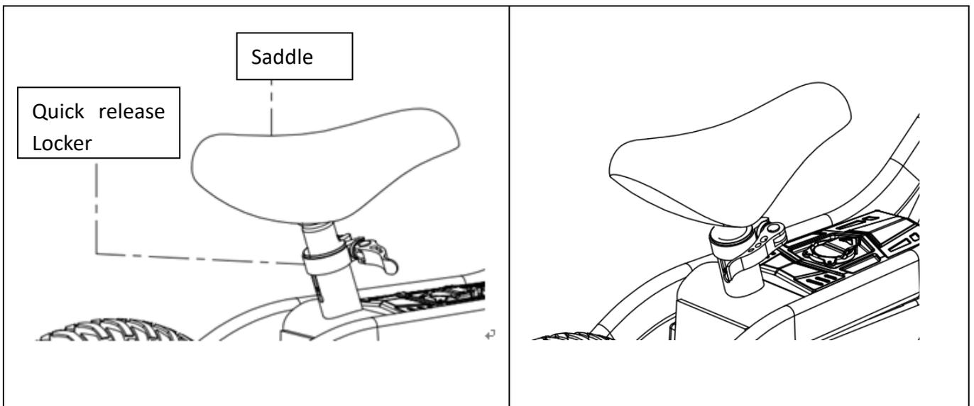
Release the lock, adjust the saddle into the right position, then lock it.
